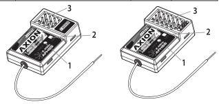
Operating Voltage: Rechargeable four to six cell NiMH, NiCd, or LiPo batteries (4.8~7.4V). From the receiver battery power or speed control (ESC) power. Select the suitable voltage depends on the servos capability. **Current Consumption: 30mA**
