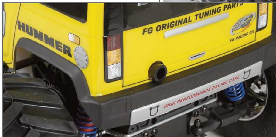
For models with bodies covering the exhaust of the silencer, f.e. Hummer and Jeep, we recommend to fix the included silicon hose at the tail pipe. Bore a whole at the respective position of the body to feed the silicon hose through it. Cut the the silicon hose corresponding to the body.
